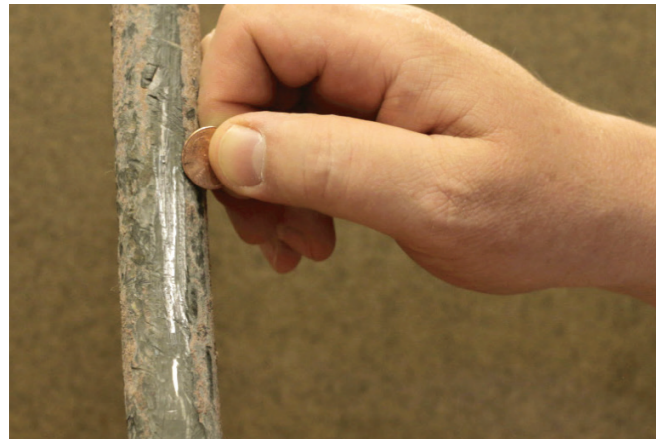
Lead Pipe If the scraped area is shiny and silver, your service line is lead. A magnet will not stick to a lead pipe.
