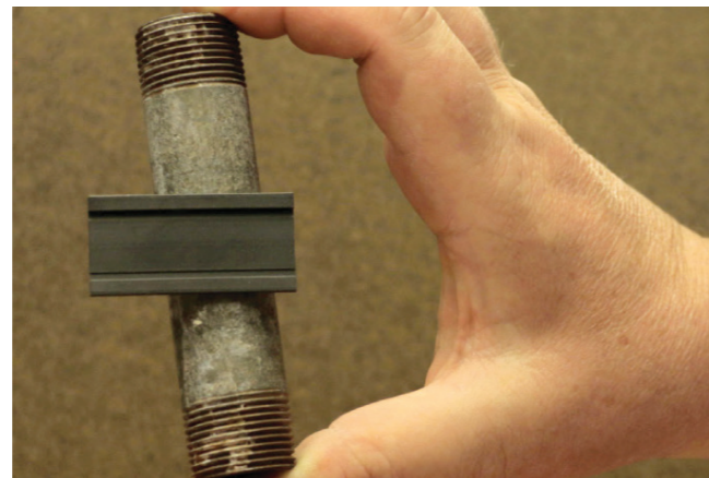
Galvanized Steel Pipe At times it can be difficult to distinguish between galvanized steel and lead pipes. If a magnet sticks to the surface, your service line is galvanized steel.
