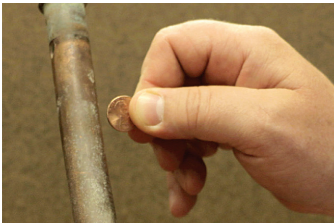
Copper Pipe If the scraped area is copper in color, like a penny, your service line is copper. A magnet will not stick to a copper pipe.
